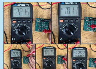
Voltage Regulation Verification
