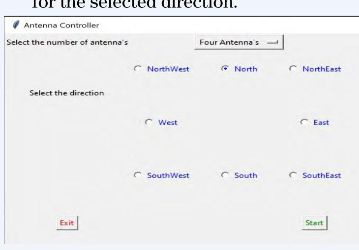
Figure 6 GUI allows user to select beam direction
