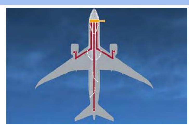
• Power distribution from the main power bus to the engine is a difficult task in modern aircraft, due to high temperatures and little free space.
