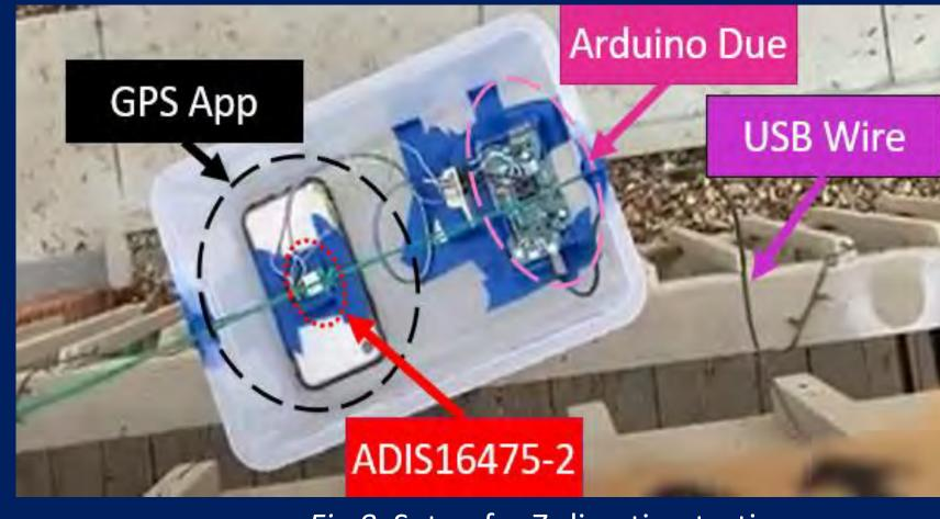
Fig 8: Setup for Z-direction testing
