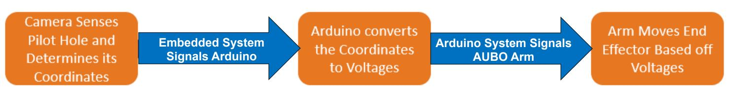
Figure 5. Overall System Diagram
