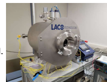
Figure 7: TVAC used for environmental testing
