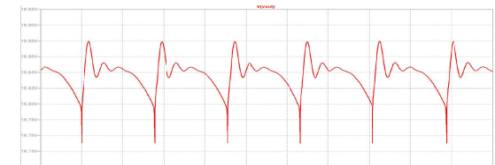
Simulated output voltage with full load (113mV ripple)
