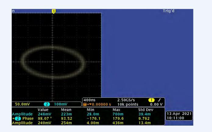
Figure 16 Phase difference between antenna 1 and antenna 2
