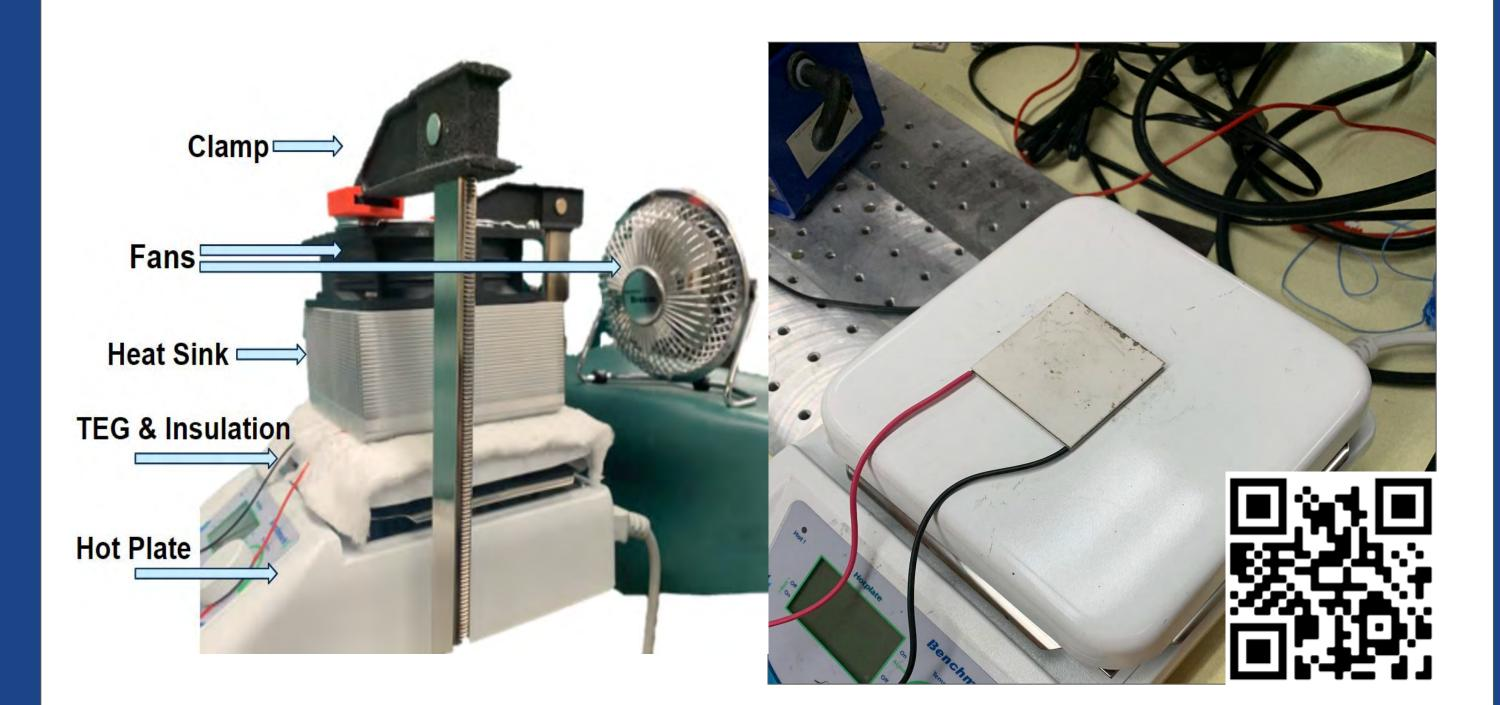
A Thermoelectric Generator (TEG) is used to harness thermal energy from a temperature gradient. To create this temperature gradient, the TEG device is placed between a hot plate and a large heatsink. The setup is pressed together using two clamps, ensuring equal force distribution and surface connection across the TEG. The hotplate is then heated up to 300°C while the heatsink is kept at room temperature.
