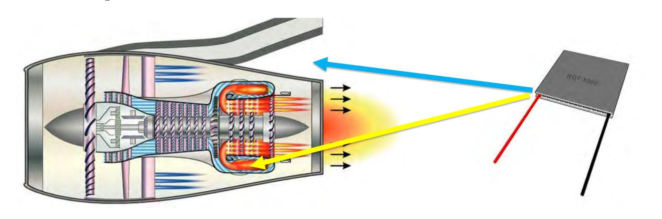
• Using a thermoelectric generator (TEG), the high temperature differential between the high-temperature core inside the engine and low temperature air outside the engine can be used to harvest energy.
