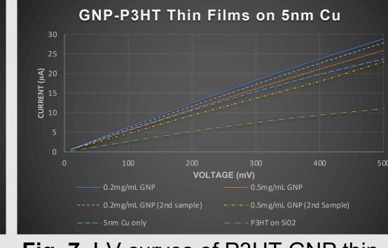
Fig. 7. I-V curves of P3HT-GNP thin films on silicon wafer with 5nm Cu layer.
