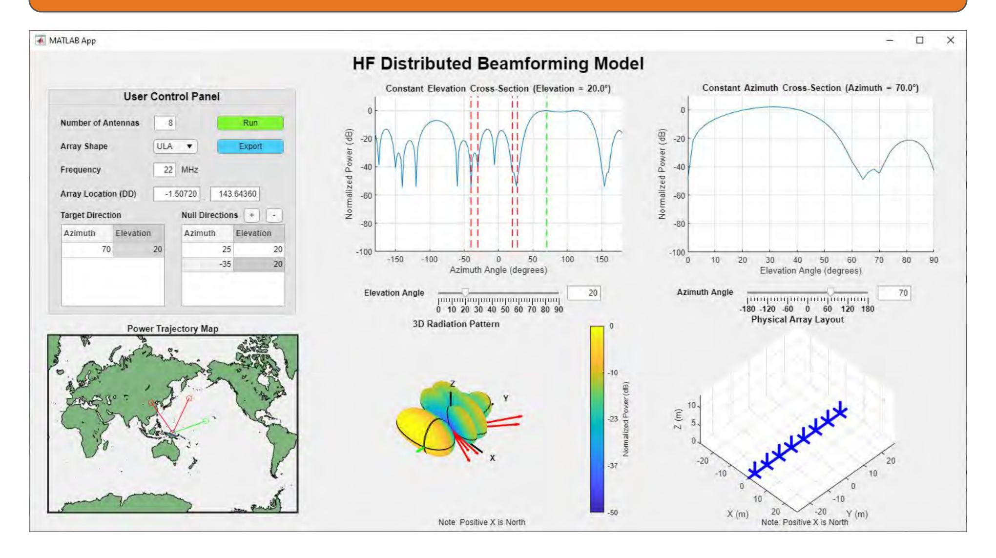
**GUI Overview:** The user inputs the target and null azimuths and elevations, number of antennas, array shape, and transmit frequency. The magnitude and phase for each antenna are computed. An internal algorithm then computes the radiation pattern and displays it.
