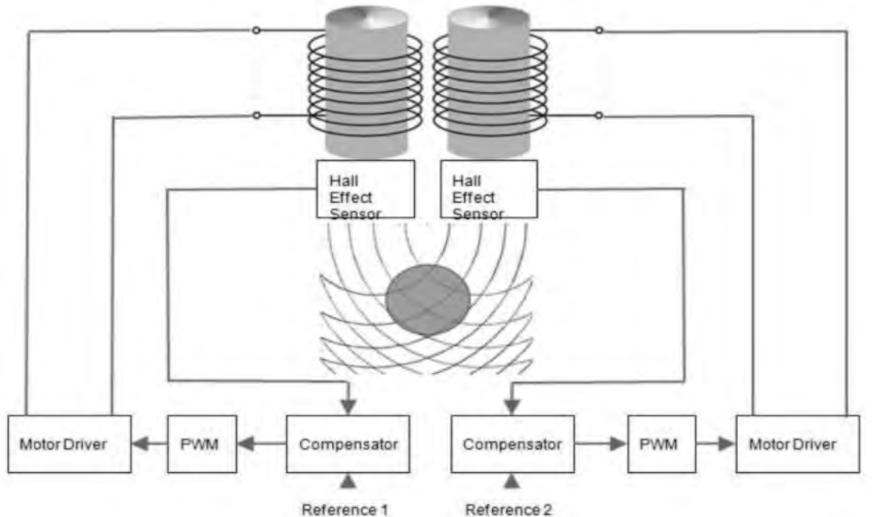
Fig 3: Horizontal movement design concept [2]
