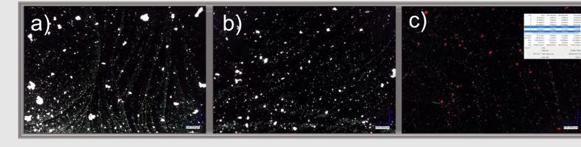
Fig. 12. GNP-Toluene thin films at: a) 1hr of sonification, b) 2hrs of sonification, c) 4hrs of sonification.
