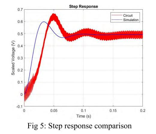
system could not achieve perfect 50% duty cycle levitation, fluctuation in the measured step response occurred. The similarities between our circuit and simulation demonstrates an understanding of the unknown plant system dynamics our designed control system achieves to levitate.
