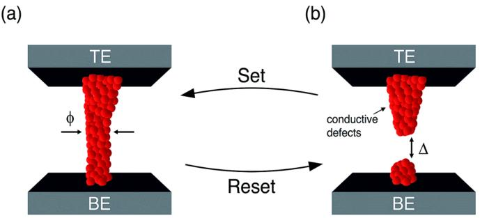
Figure 2:ReRAM Cell Switching
