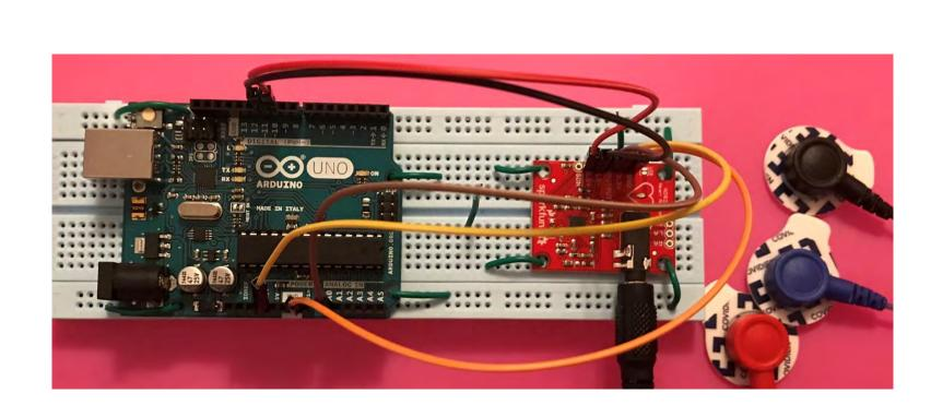
ECG Arduino Circuit
