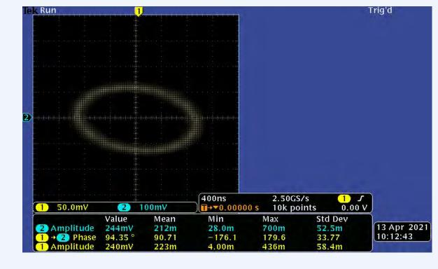
Figure 18 Phase difference between Port 1 and Port 4
