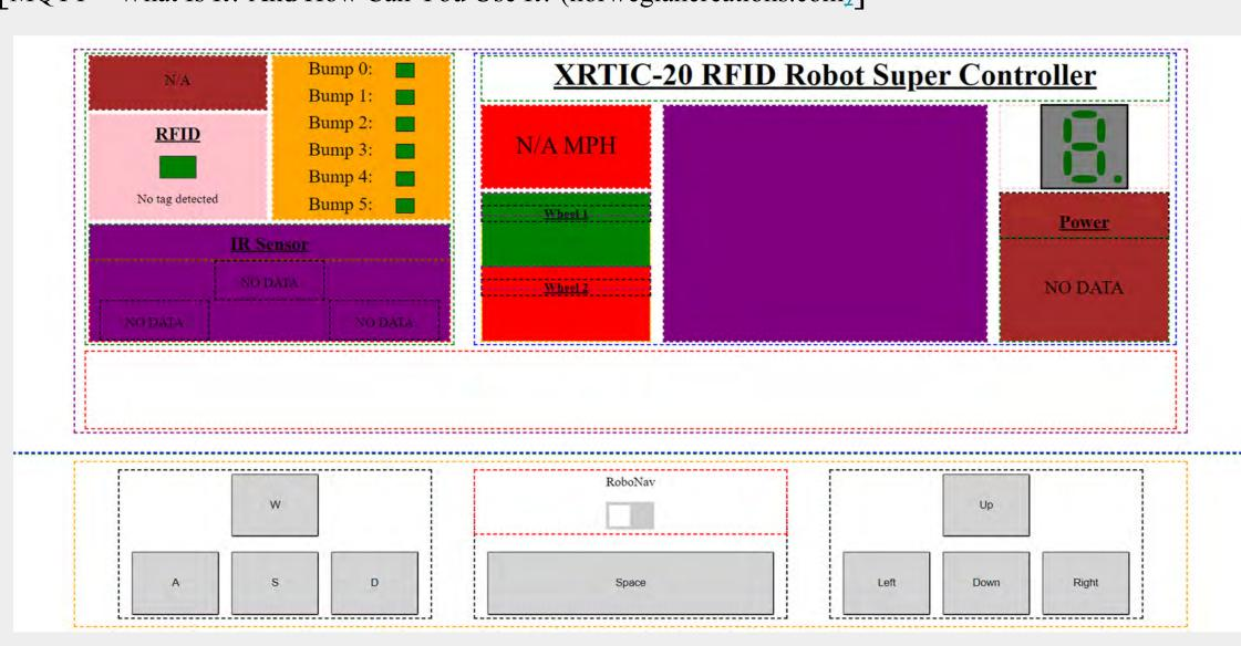
Our HTML based controller, which sends commands over MQTT
