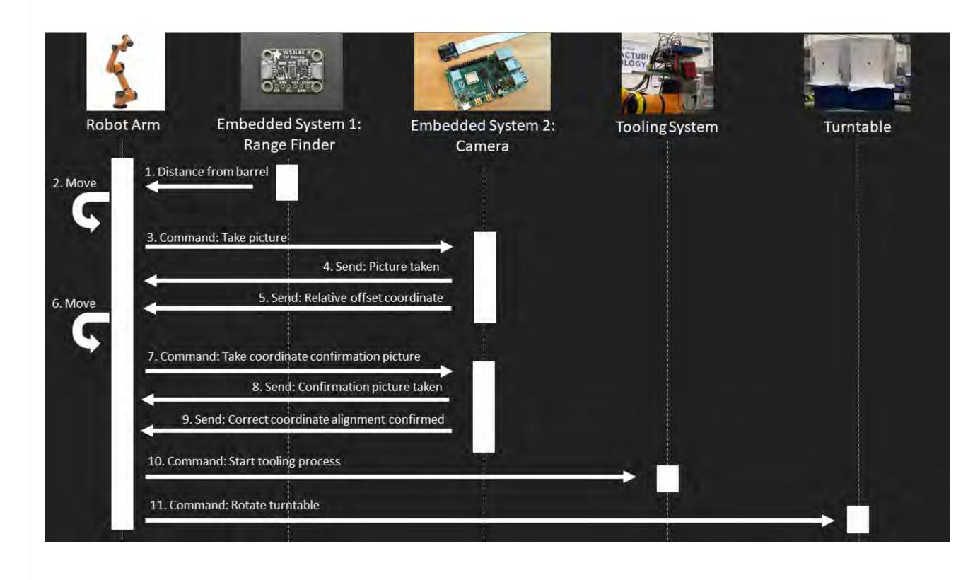
Figure 1. Sequence Protocol Diagram
