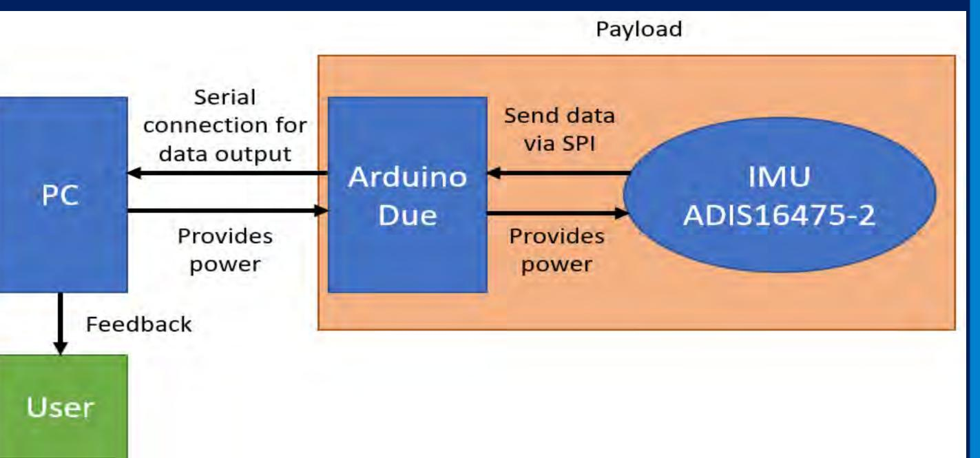
Fig 2: System Context Block Diagram
