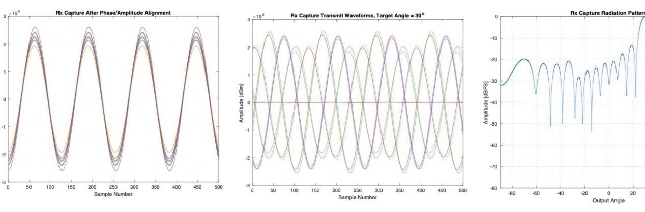
Figure 6. Rx capture following phase and amplitude system alignment
