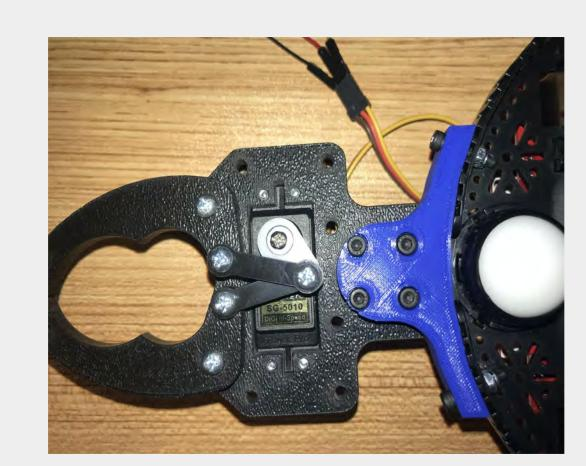
A simple, single degree of freedom, two-fingered gripper. We designed 3D a printed strut to attach the gripper to the chassis.
