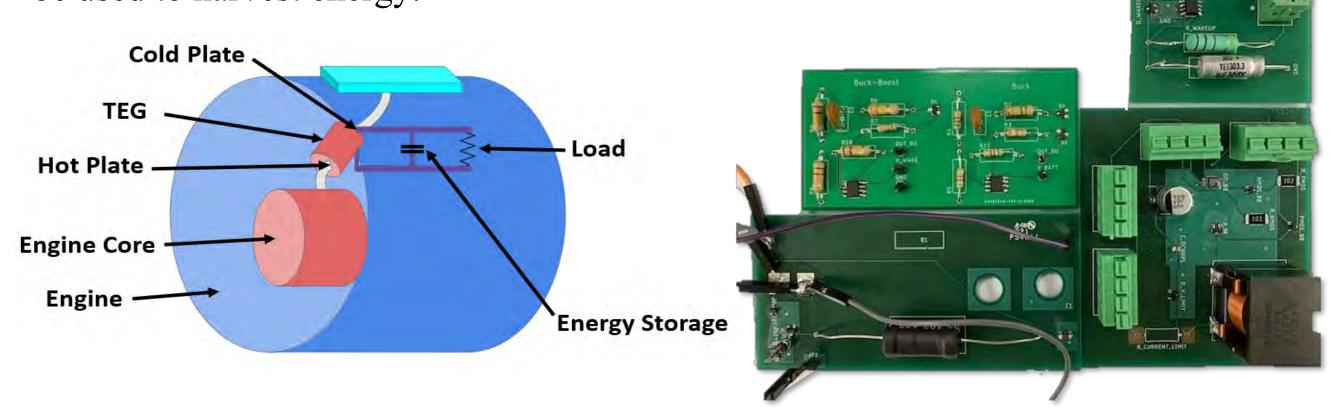
• Implementation of an energy harvesting and storage circuit will allow for maximum power transfer from the TEG, and ensure reliable delivery of power to the sensor.
