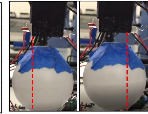
Fig 11: Horizontal movement of a two-solenoid system using analog circuit theory
