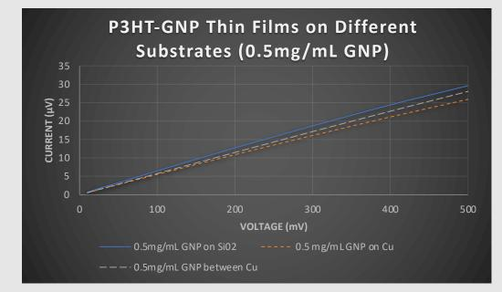
Fig. 14. I-V characteristics of P3HT-GNP thin films on multiple substrates with 0.5mg/mL GNP.
