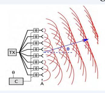
Figure 3 Visualization of beam steering through phasing.
