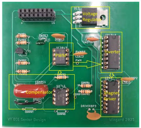
Figure 5: Analog Controller PCB The design was tested on a breadboard, then translated to a PCB for the final product. Each magnet in the array is controlled by a single controller. To allow for user controls, the bias voltage of each controller was supplied by DACs (MCP4822) controlled by an Arduino Mega 2560. Click here to see the analog controller's tracking ability.
