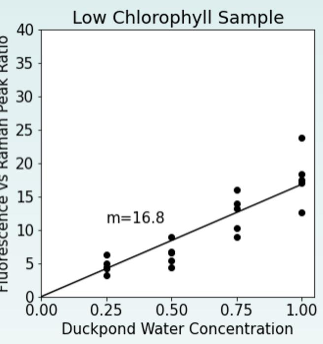
Plots showing linear relationship between chlorophyll levels in water and measured peak ratio between 685 nm (chlorophyll peak) and 527 nm (raman peak)
