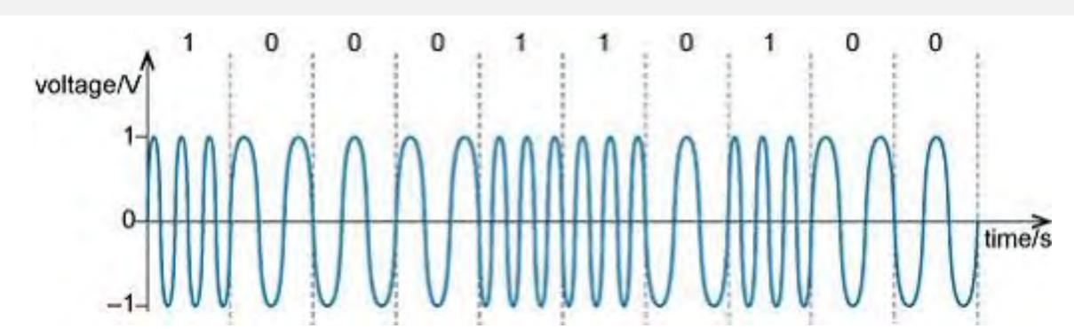
Frequency Shift Keying Diagram [1]. Different bits (or groups of bits) are encoded as different frequencies.
