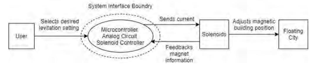
Fig 2: High level realization of microcontroller control design
