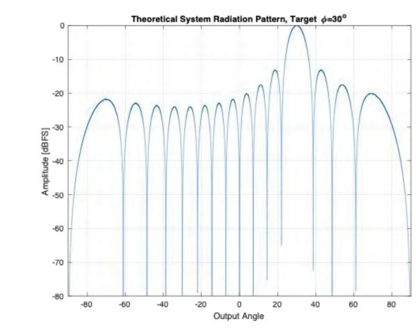
Figure 5. Theoretical calculated beam pattern.
