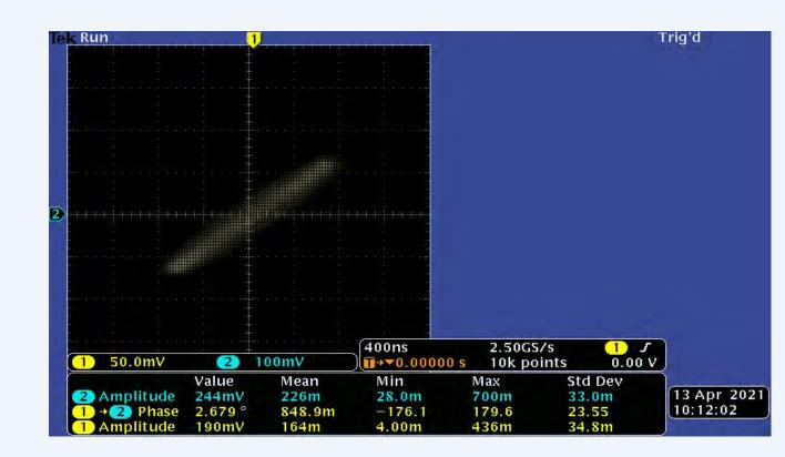
Figure 17 Phase difference between antenna 1 and atennat 3
