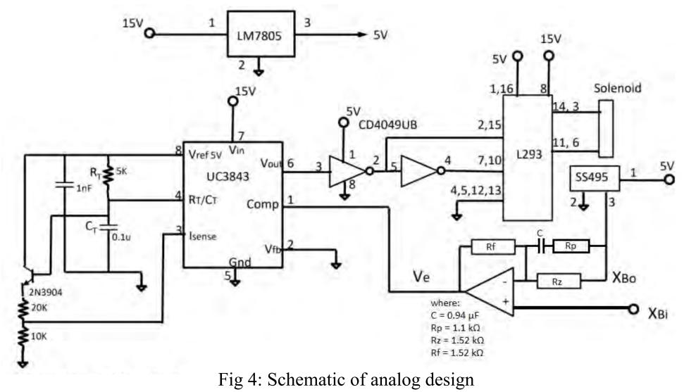
By researching the levitation problem as the control of a naturally unstable system, our compensator for the above schematic was designed about controlling this theoretical unstable system. Fig 5 shows the found compensator step response compared with the theoretical response. Since the
