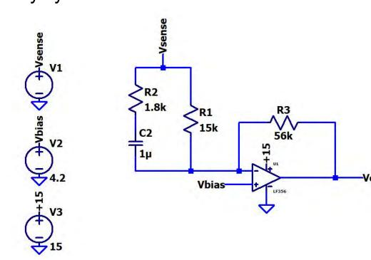
Figure 3: Analog Compensator Design
