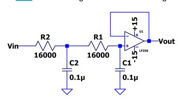
Figure 6: Second Order Low Pass Filter
