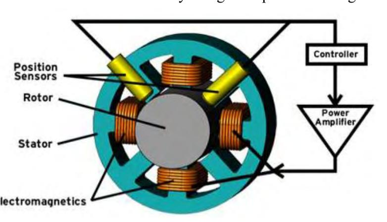
Fig 1: Magnetic bearing example showcasing use case of magnetic levitation [1]
