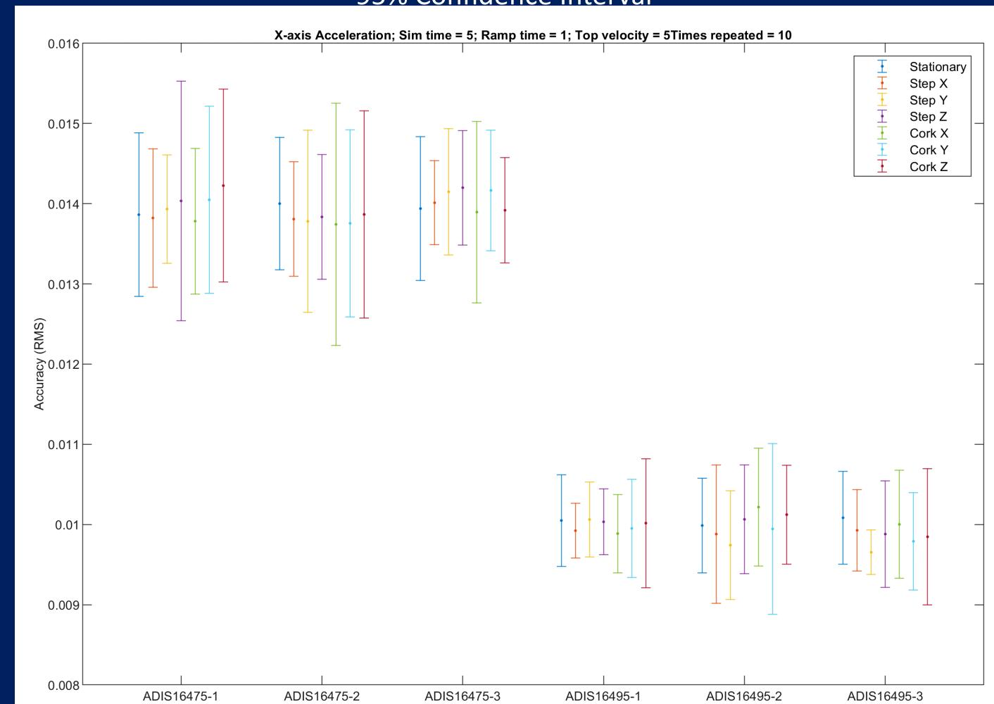
Fig 5: Confidence intervals for all seven simulations and all IMU models. Tests were run 10 times to generate a median RMS values and confidence intervals.
