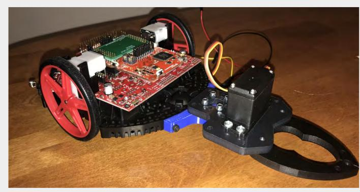
Gripper is mounted on the rear of the rover to the chassis, which powered by a servo, which can be set to different positions by varying the pulse width of its input signal.
