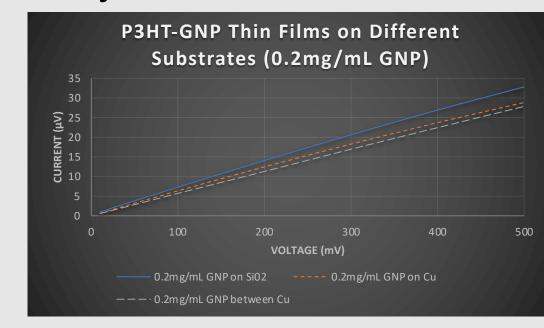
Fig. 13. I-V characteristics of P3HT-GNP thin films on multiple substrates with 0.2mg/mL GNP.
