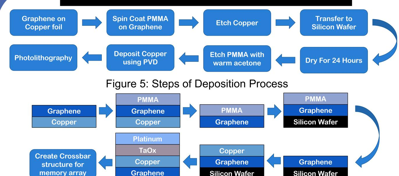
Figure 6: Process of Building ReRAM Memory Array
