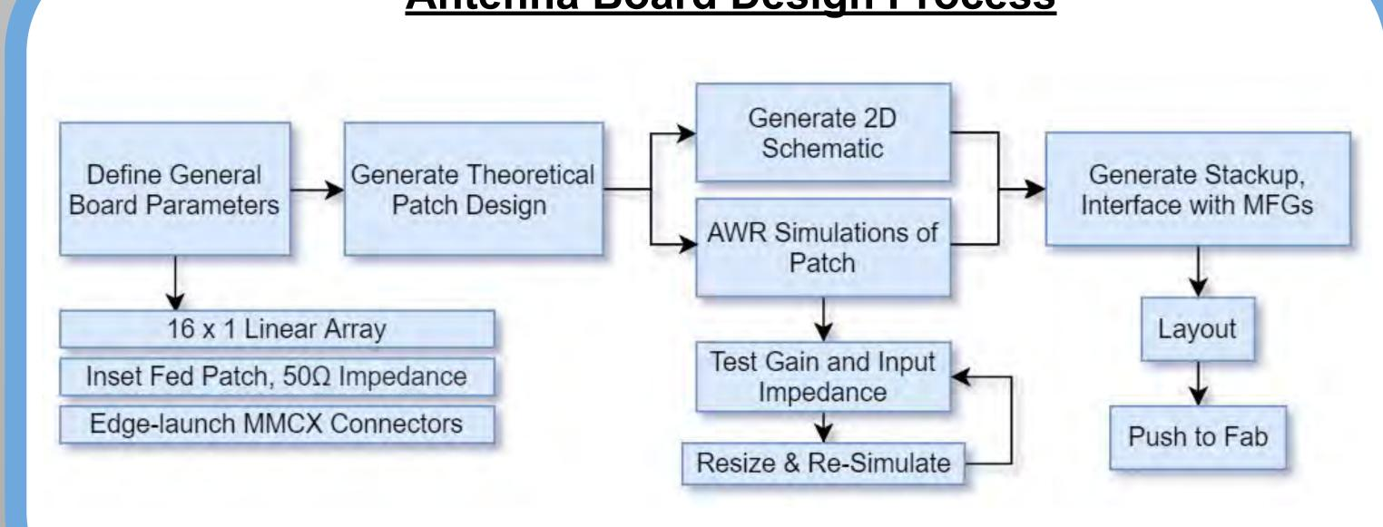
Figure 9. Antenna board design process.
