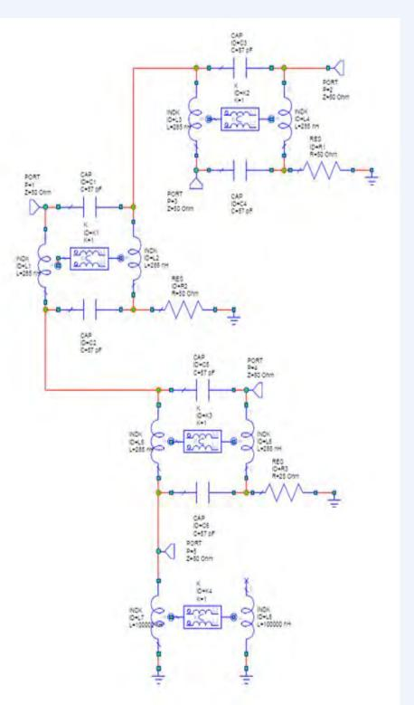
Figure 11 Schematic for Phasing Circuit
