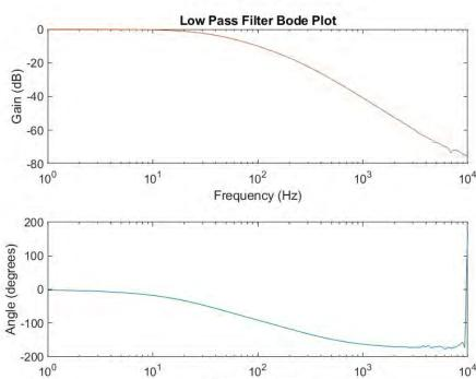
Figure 7: Low Pass Filter Bode Plot
