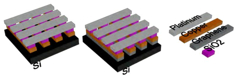
Figure 3A: ReRAM memory array B: Graphene Enhance ReRAM C: Key
