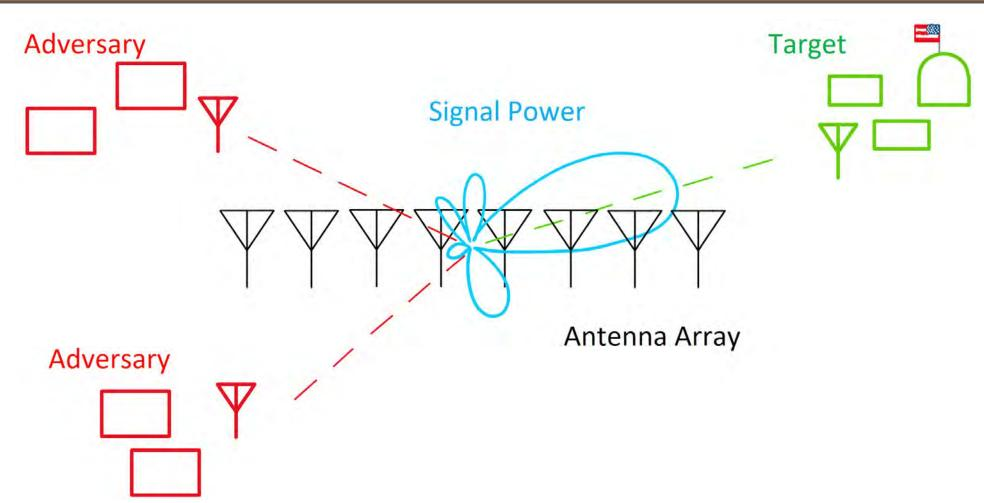
In the image above, the antenna array directs power towards the target receiver and minimizes power in the directions of the adversaries. The signal strength in a given direction is represented by the blue beam pattern's distance from the center of the array.
