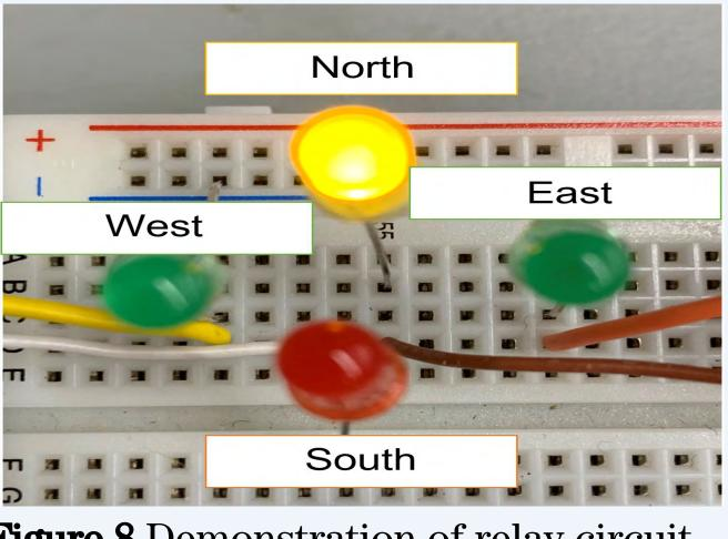
Figure 8 Demonstration of relay circuit with leds
