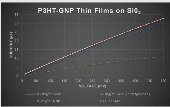
Fig. 6. I-V curves of P3HT-GNP thin films on silicon wafer with Si02 layer.
