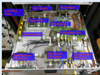
Figure 3: Labeled image of a transmitter at the Blackstone, VA site
