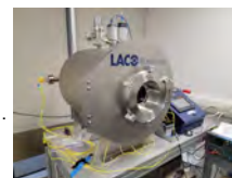
Figure 7: TVAC used for environmental testing
