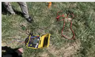
Soil Resistance Testing in North Field
