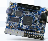
DE10-Lite Developer Board with MAX 10 FPGA
