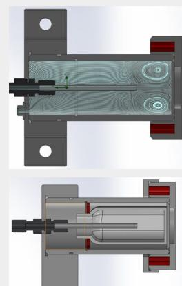
*Customer's Current Accumulator Design and its Flow*
