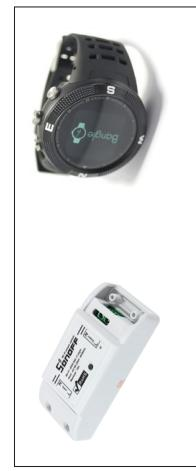
**Figure 3:** The device on the left is the Sonoff control switch used to control externally connected smart devices all over Wi-Fi. The device is used to toggle control of a light based on events triggered by sensor data from the watch. The device on the right is the Bangles smart watch which is the physical fitness watch used in this project to demonstrate the full functionality of an interface based on Open Sound Control and which is controlled by sensory inputs from a human user.
