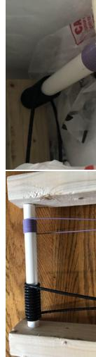
Left: Cables secured around a 1/4 inch mandrel. Right: cables after 24 hours exposed to dry ice
