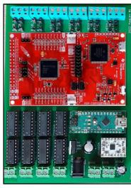
Fig: MSP432P018, used for digital control
