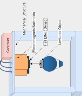
The control loop is duplicated for each solenoid and run in parallel to achieve multi-solenoid control. Horizontal movement is achieved with out-of-phase sinusoidal setpoints.
