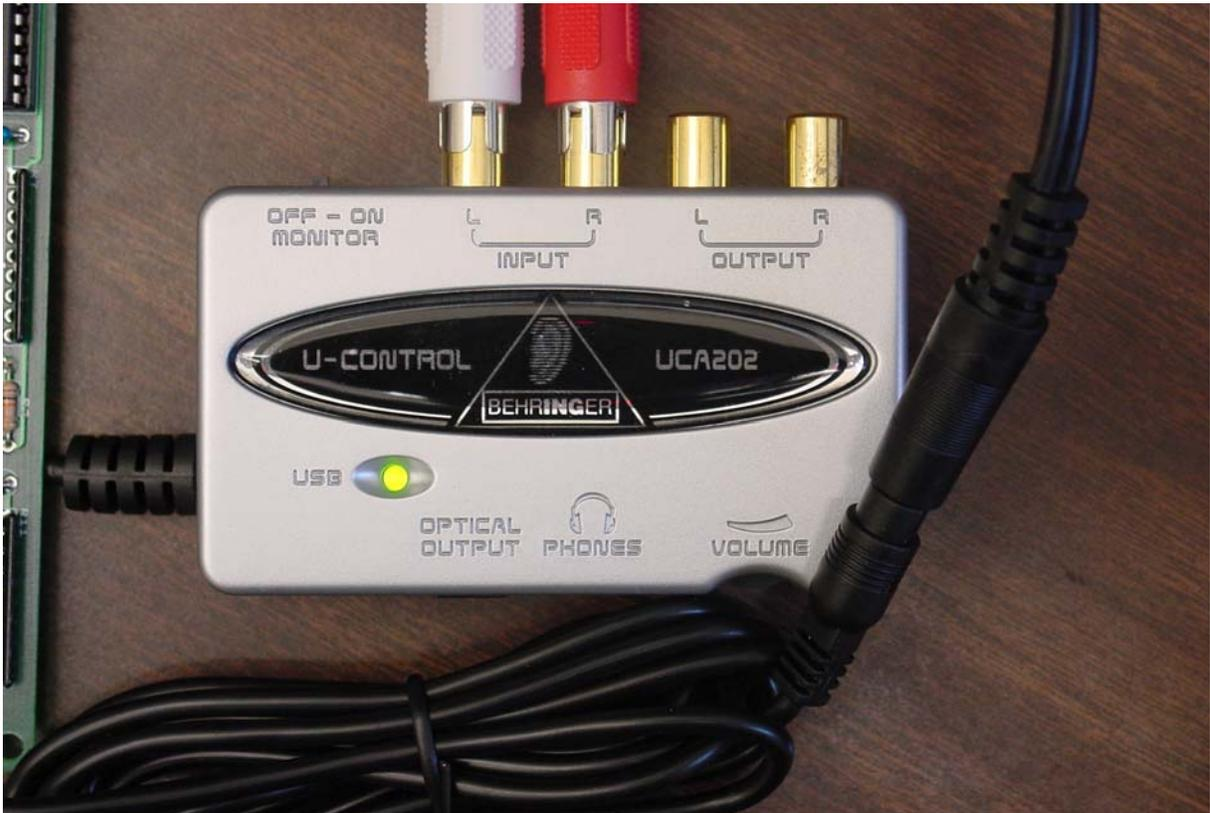
Figure 3: Connecting cables to the UCA202
